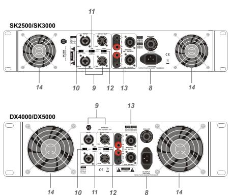
**8. AC input socket:** Standard 3PIN IEC power connector, which connects to main power network through attached power cable. Please make sure the power is right before connecting to voltage.
